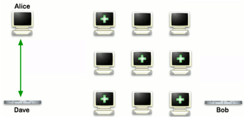
Figure 1: Alice’s OP obtains a list from a directory server. The pluses symbolize ORs commonly run by volunteers.
